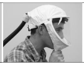
5. With the breathing hose connected, slip the headgear over your head with the elastic area under your chin. Tighten the headgear ratchet to a snug and comfortable fit if necessary. There should be no gaps between head cover and face. Readjust headgear if gaps are present
