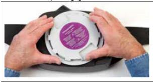
8. Insert the filter evenly into the filter pocket. Lock the filter by turning it clockwise 90 degrees until you hear a "click" and filter icons are aligned Filter should sit level with the top of the blower unit. Filters cannot be overtightened
