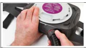
12. Lock the breathing tube by rotating the connector clockwise 90 degrees until it locks in place. Once installed, pull gently on the hose connector to verify it is secure
