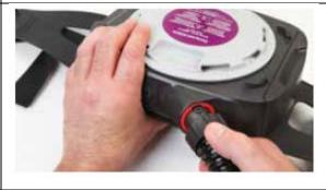
11. Insert the breathing tube blower-side connector to the red port on the top of the blower by lining up the posts on the connector with the notches in the port
