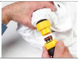
19. Connect the breathing tube to the air duct connector and twisting it clockwise until it locks. Once installed, pull gently on the hose connector to verify it is secure
