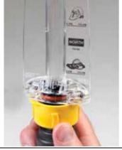
14. Insert the free end of the breathing tube into the flow indicator as shown above. Keep the flow indicator level and ensure the ball is above the line marked 6 cfm (170 lpm)
