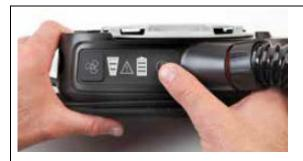
1. Turn off PAPR by pressing and holding the power button for 3 seconds until the unit emits a beep and powers down
