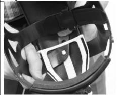
17. If further adjustment is needed, release the two straps from the yellow locking pin and move straps and align to desired Small, Medium, or Large holes and snap them back into the locking pin. Tuck ends of strap back under yellow air duct attachment
