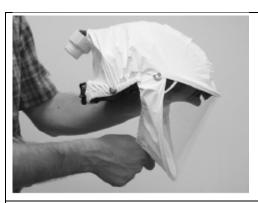
18. Slip head cover over headgear. The top opening in the head cover will go over the yellow hose connector on the air duct. Pull yellow hose connector through head cover. Elastic strap should be placed under the ratchet. Snap head cover onto the headgear. Remove protective lens covers (inside and outside) of the head cover before using the respirator
