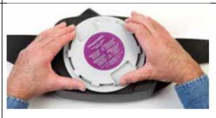
4. Remove filter by rotating counter-clockwise. If at end of filter life discard via local and EPA regulations. If filter can be reused, place in resealable container
