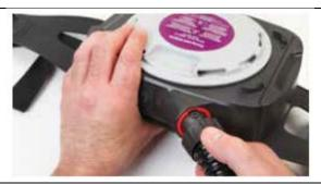
7. Disconnect breathing tube by rotating the blower side connector counter-clockwise 90 degrees until it releases
