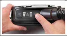
13. Ensure the filter is installed and the headpiece is NOT connected. Press and hold the round power button for 3 seconds until the unit begins its power-on sequence. LED lights should flash and the unit will emit an audible beep and vibrate
