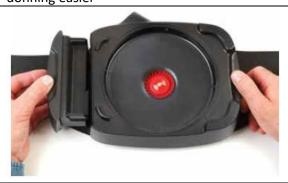
5. Remove the battery from blower. Grip battery while pressing latch button and pull battery out
