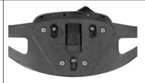
6. Remove blower assembly from harness. Lift up on latch in center of harness and slide the blower toward the open end of keyholes
