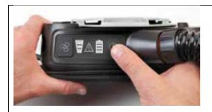
4. If not already done, turn PAPR on by pressing the round power button for 3 seconds until the unit begins its power-on sequence. LED lights should flash, the unit will emit an audible beep and vibrate
